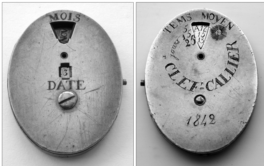
Fig. 1. The Clef-Callier showing (left) the month and day and (right) the Equation of Time on the reverse.
