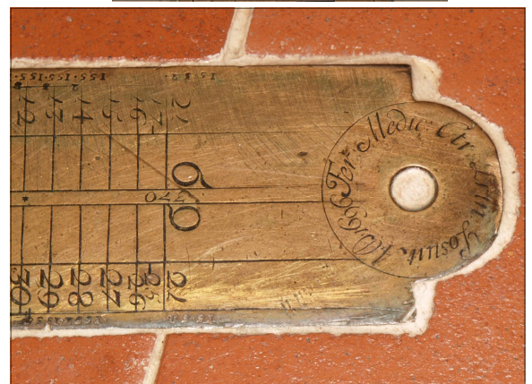
Fig. 6 a, b. Detail of the parts of the sundial referring to the winter and summer solstices.
